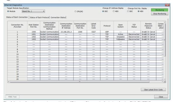
The following functions can be used in the "Ethernet Diagnostics" window for the FX5-ENET/IP.
