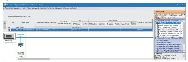
Drag and drop an "Ethernet Device" in the "Module List" to the left side of the screen, and set the following items. The setting items vary depending on the "Ethernet Device" and "Communication Method".
